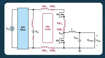
Figure 1. A buck converter with Hot Loop ESRs and ESLs.
