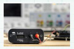
Figure 1: Otii Arc delivers the power profile of low-power and battery-powered applications. Using scripts, tests can also be automated. Source: Qoitech AB. (NOTE: source - https://www.qoitech.com/wp-content/themes/ yootheme/cache/9f/lab\_-scaled-9f26da9b.webp).
