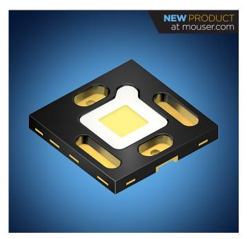
OSLON 5-Chip Black Flat X KW5 HQL631.TK LEDs highperformance are the most efficient lead-frame devices in the OSLON series, delivering exceptional performance in automotive exterior applications, including halogen replacement. The high-efficiency LEDs offer up to 2140 lm at 1000mA, and they boast an operating temperature range of -40°C to +135°C.
