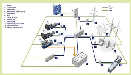
Figure 2: A typical microgrid arrangement in a factory environment. (Image reproduced with the permission of Rolls-Royce Power Systems AG
